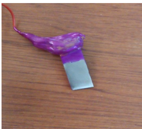
Figure 2: Sample preparation for OCP experiment.
