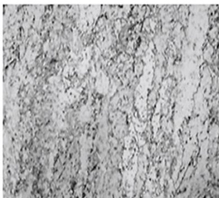
Figure 4: Micrograph of as-received Ti Grade 2 material, 100X.
