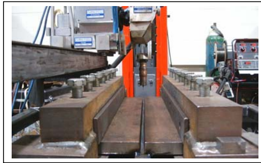
Figure 1: plate jig of narrow groove plate weld.
