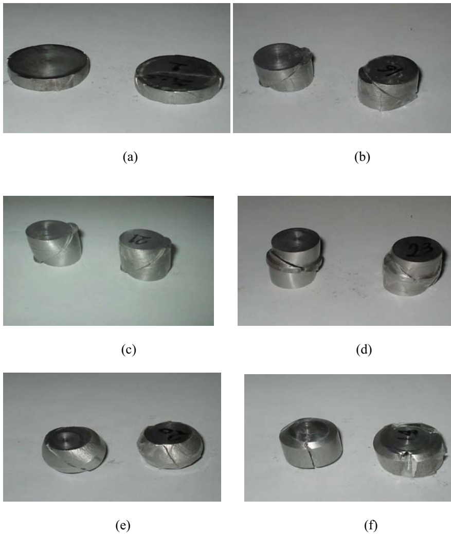
Figure 10: Fractures on the surfaces of compressed Al-based alloy specimens
