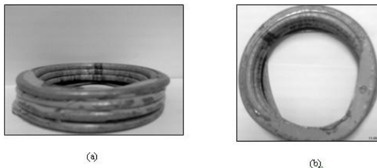
Figure 7: Extensional collapsed mode. (a) Front view. (b) Top view
