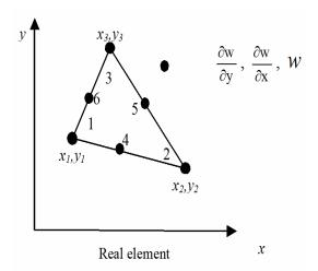
Figure 6: six nodes eighteen degrees of freedom triangular element
