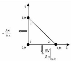
Figure 5: Parent elements normal derivatives
