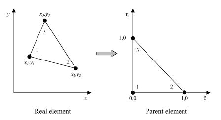
Figure 1: Parent and real triangle elements
