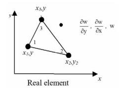
Figure 3: three nodes nine degrees of freedom triangular element
