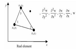
Figure 4: three nodes eighteen degrees of freedom triangular element
