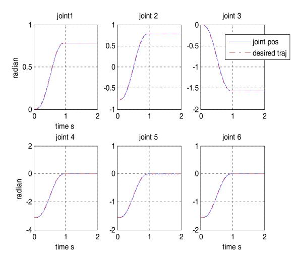
Figure 3a: IRp-6 joint position tracking under constrained linear CTC-PD controllers
