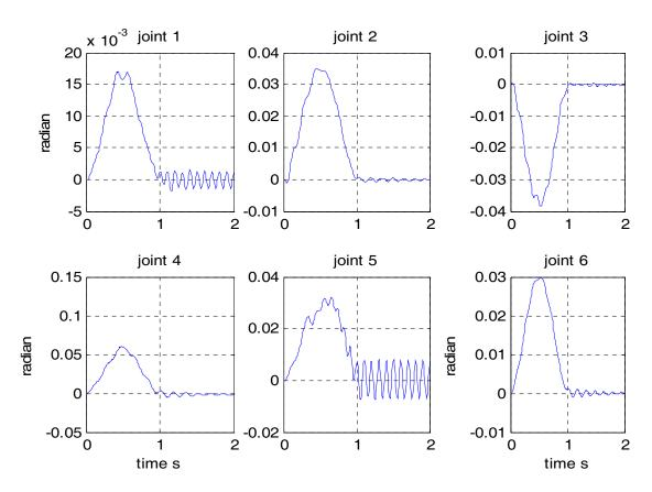
Figure 3c: IRp-6 joints position error under constrained linear CTC-PD controllers
