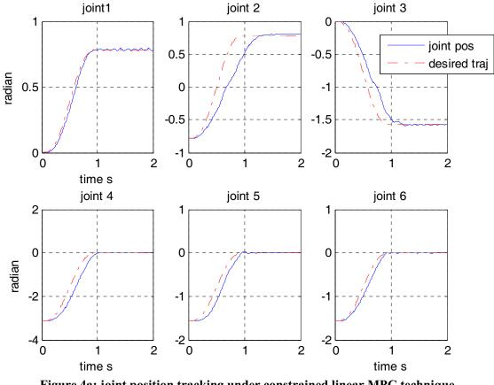
Figure 4a: joint position tracking under constrained linear MPC technique
