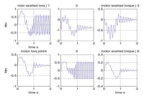
Figure 3b: IRp-6 joint motor torque under constrained linear CTC-PD controllers
