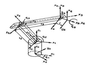
Figure 1: Free-body Geometric structure of the Irp\_6 Robot
