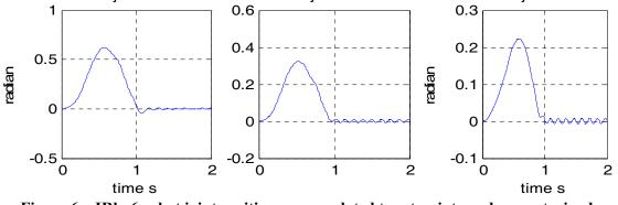
Figure 6c: IRb\_6 robot joint position errors related to set-points under constrained hybrid controller
