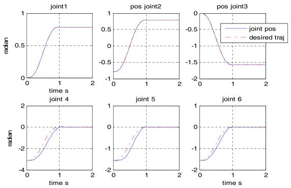
Figure 6a: Joints positions of IRp\_6 robot under constrained linear hybrid controller
