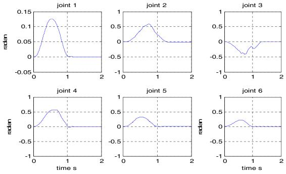
Figure 4c: Joint position tracing error torque under constrained linear MPC technique
