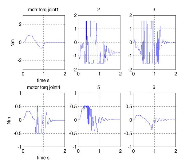
Figure 4b: joint motor exerted torque under constrained linear MPC technique
