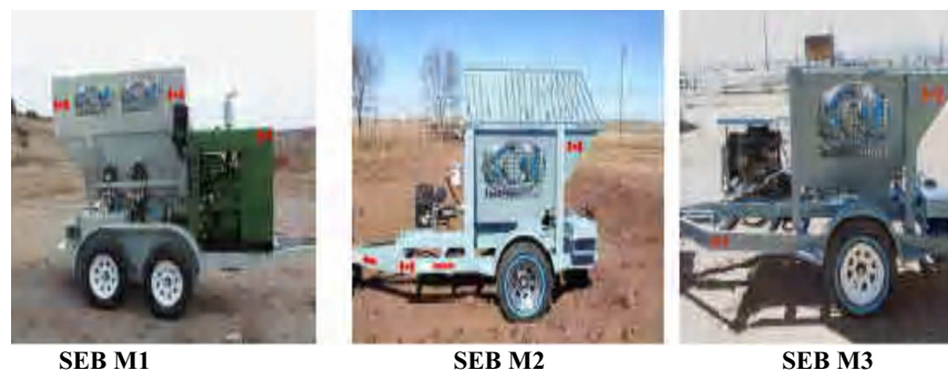
Figure 3: Three types of Stabilized Earth Brick (SEB) Machines which can be easily transported on to a construction site.
