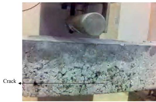
Figure 3: Crack formation in a 50% EPS Specimen
