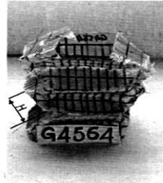
Figure 9: Developed view of the tube deformed as above
