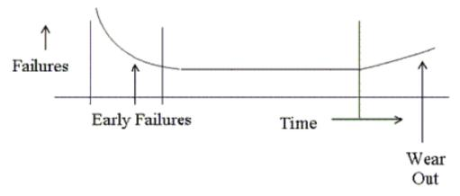
Figure 1: Typical Electronic Component Failure Rate as a Function of Age [7].
