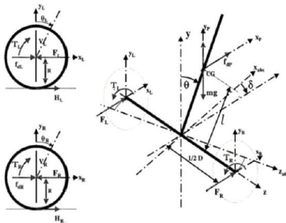
Figure 1: Diagram of forces and moments acting on the TWIPMR system
