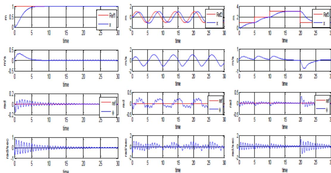
**Figure 7: Simulation results of FLC for neuro model of TWIPMR**
