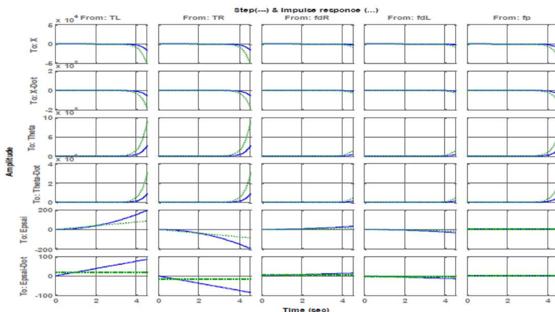
**Figure 3: Open loop unit step and impulse response of the transfer matrix**
