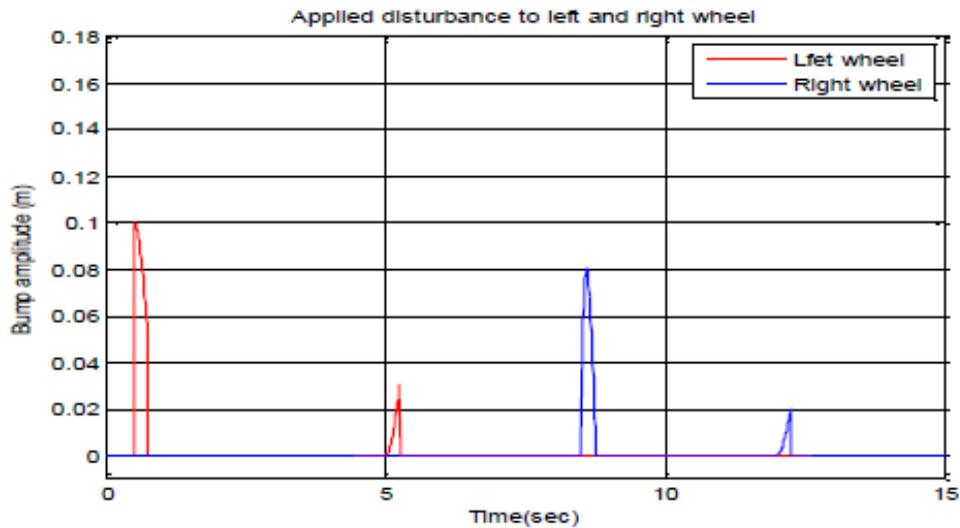
**Figure 17: Profile of left and right wheel disturbance**
