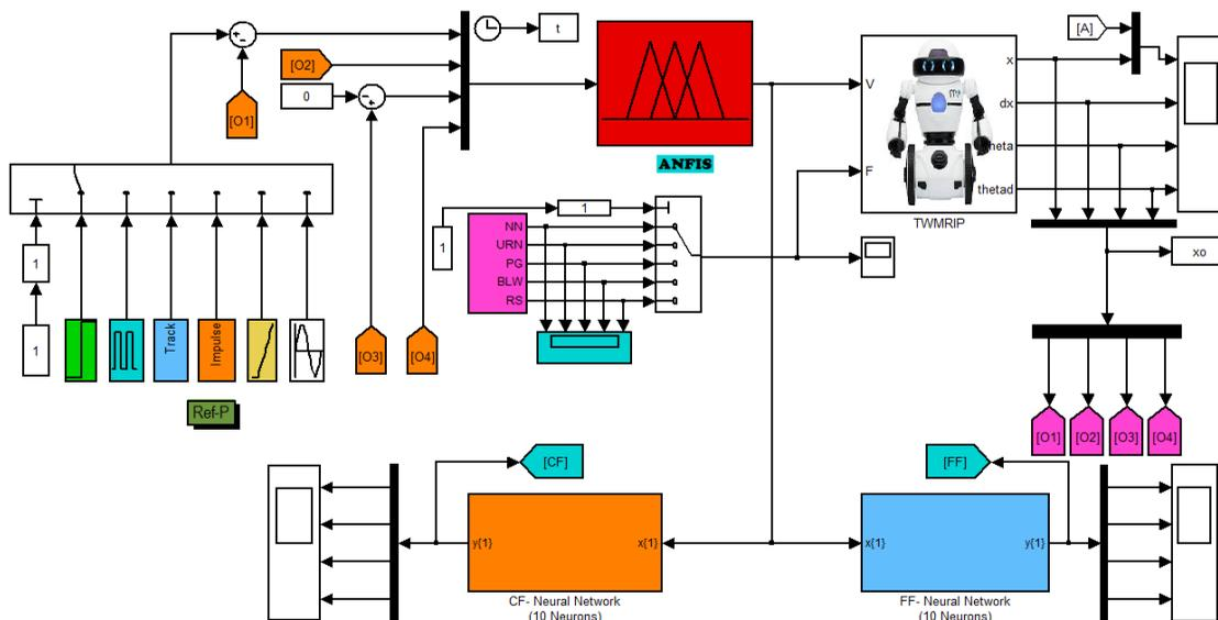
**Figure 12: Simulink model of TWIPMR using neuro-fuzzy scheme**
