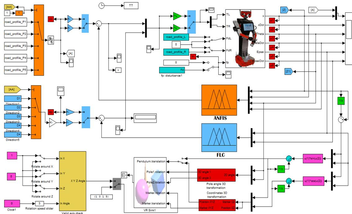
Figure 15: The link between Simulink model and virtual world
