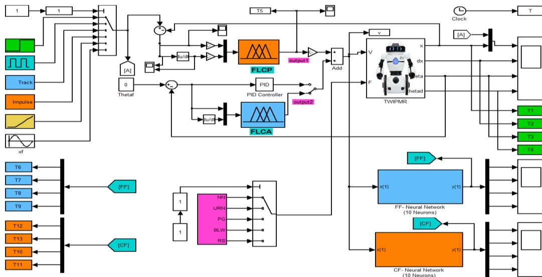
Figure 4: Simulink model of actual and neuro model with Fuzzy Logic Controller
