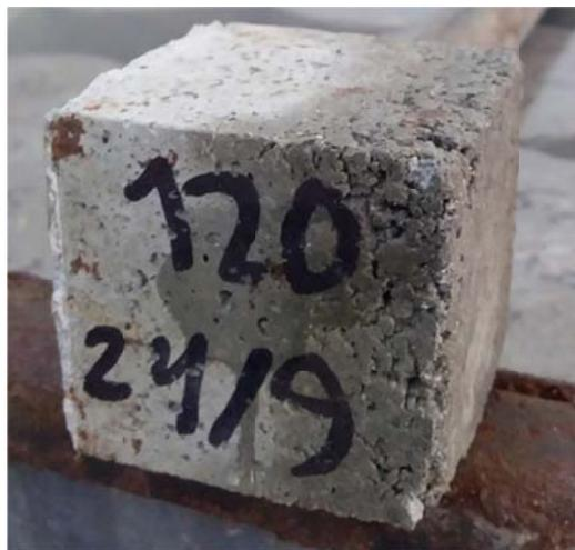
**Figure 10: Illustration of voids in MC3 mixtures made without addition of HRWRA**
