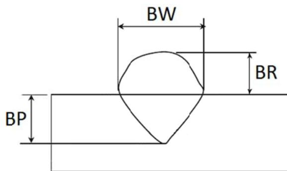
**Figure 1: Weld bead parameters**
