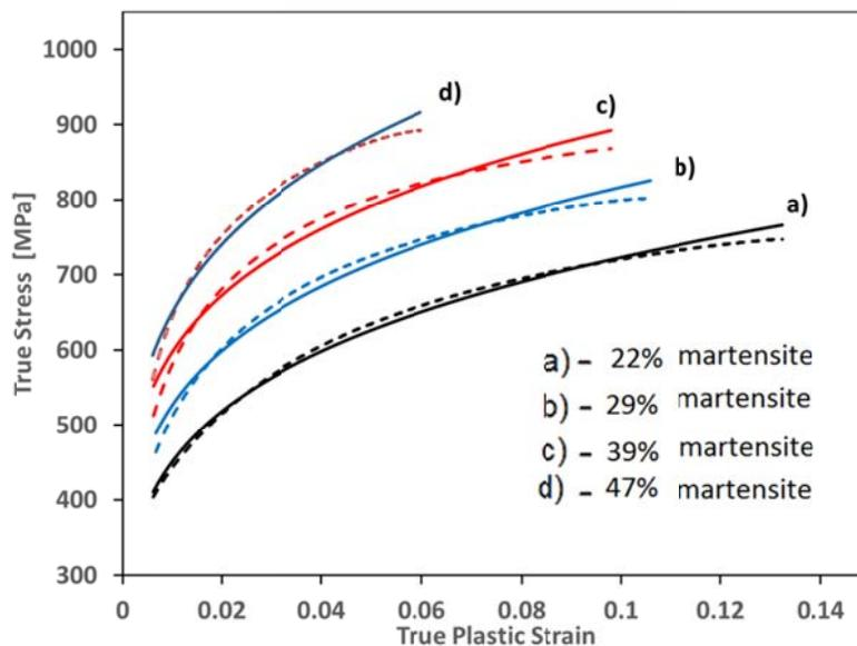
**Figure 3: Correlation between the experimental true stress-true plastic strain curves for dual phase steel with different volume fraction of martensite (broken lines) and the corresponding theoretical ones calculated according to the Hollomon's model (solid lines)**
