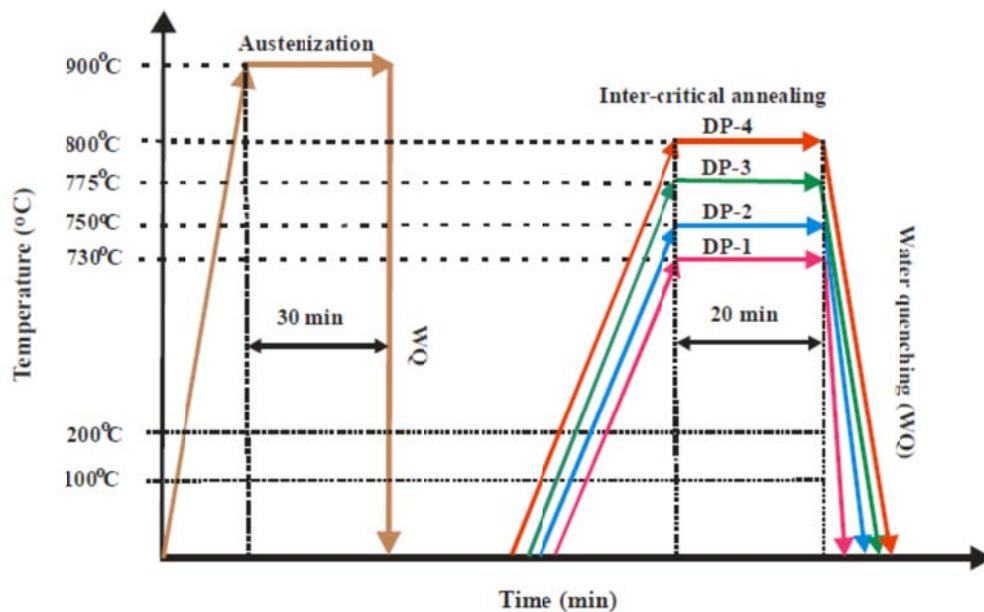
**Figure 2: Schematic drawing of heat treatment cycle used in this investigation**
