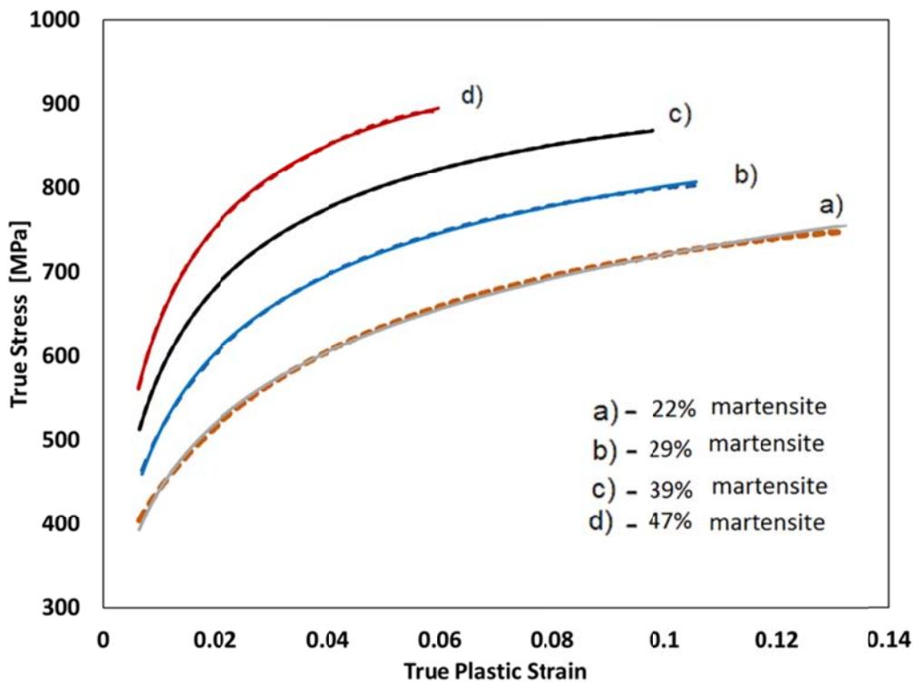
**Figure 5: Correlation between the experimental true stress-true plastic strain curves for dual phase steel with different volume fraction of martensite (broken lines) and the corresponding theoretical ones calculated according to the Log-Method's model (solid lines)**
