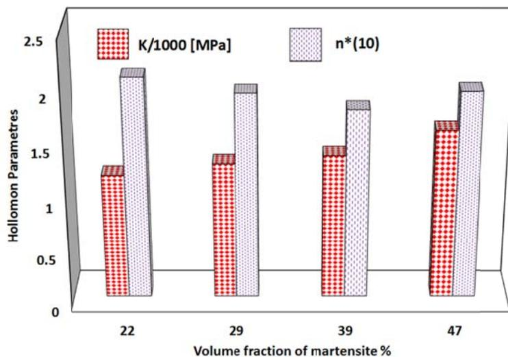
**Figure 4: Effect of volume fraction of martensite on Hollomon parameters**
