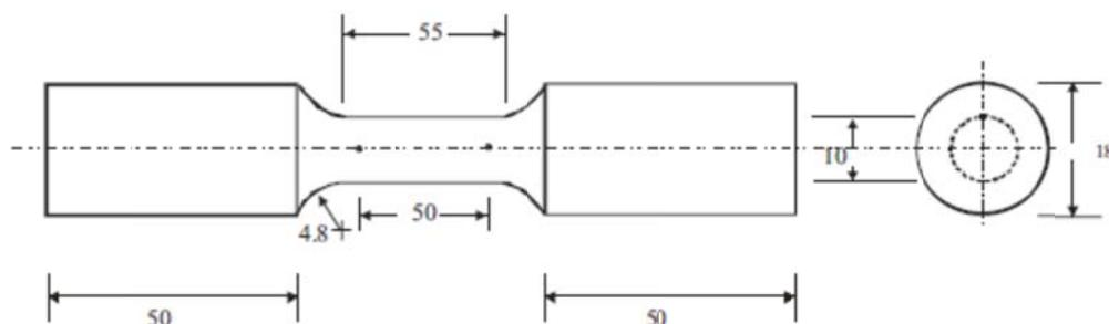
**Figure 1: Dimensions of the tensile test specimens (in mm)**
