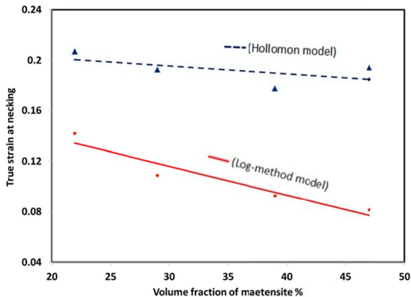
Figure 8: True strain at necking instability as a function of the volume fraction martensite.
