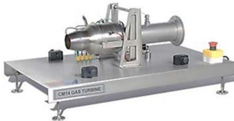
**Figure 1: CM14 Turbojet engine [2].**
