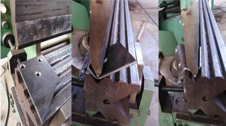
**Figure 14: Bending the sail tie with the press machine.**
