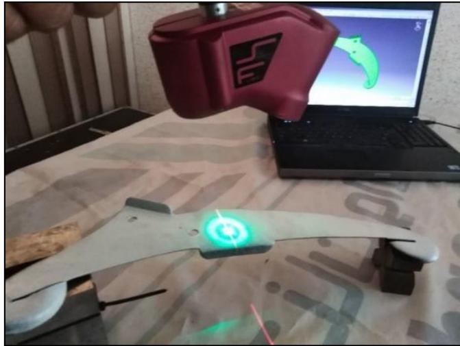
**Figure 4. Baces3D arm during scanning of the rib.**
