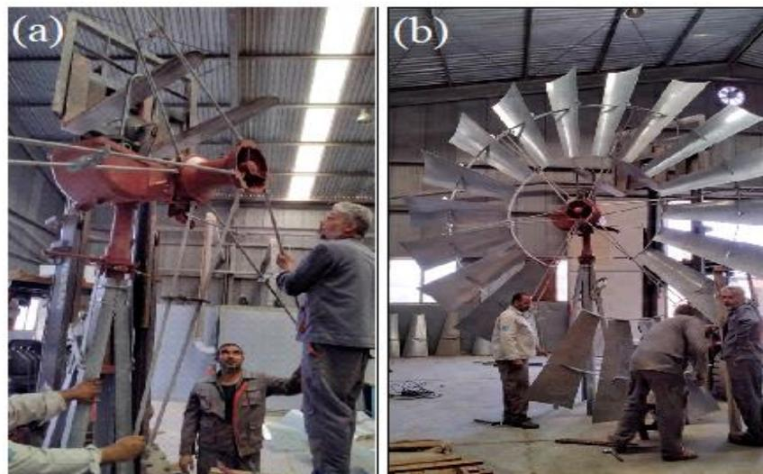
Figure 17. (a) Installing rotor arms into hub; (b) Assembly of the 6th sails section.
