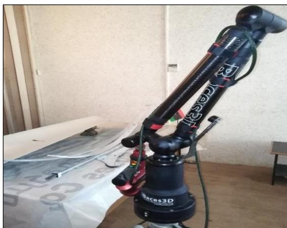
**Figure 2: Baces SCAN portable laser scanning system.**
