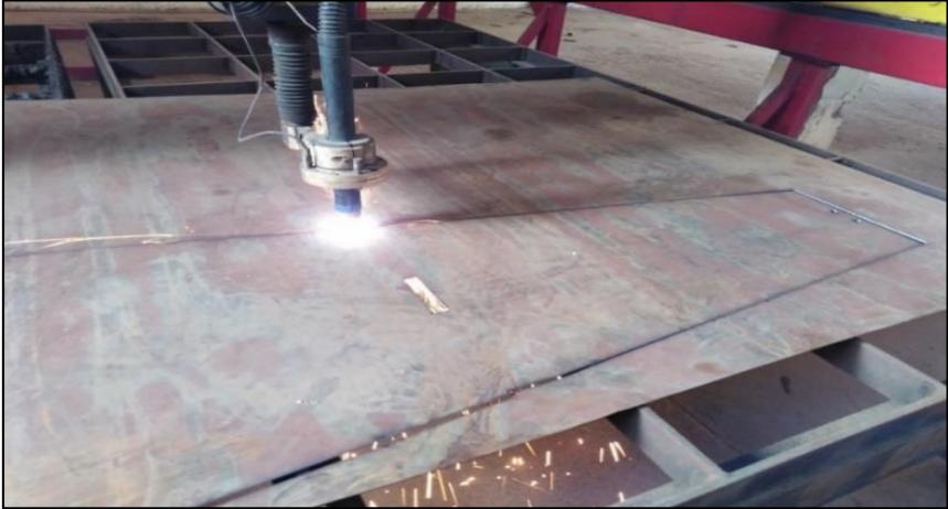
**Figure 13: Sails cutting with a CNC plasma machine.**
