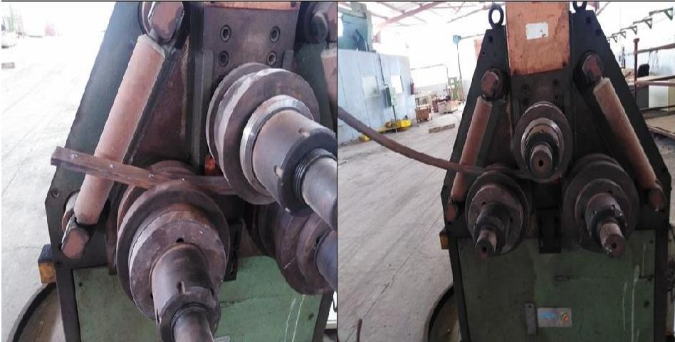
**Figure 15: Using a CNC rolling machine to bend the outer band**
