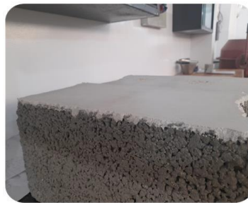
Figure 7: Test specimen capped according to the ASTM-C1552 standard.
