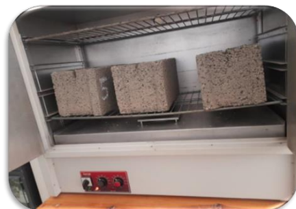
Figure 6: Specimens dried in an oven at a temperature of 100°C to 115°C for 24 hours.
