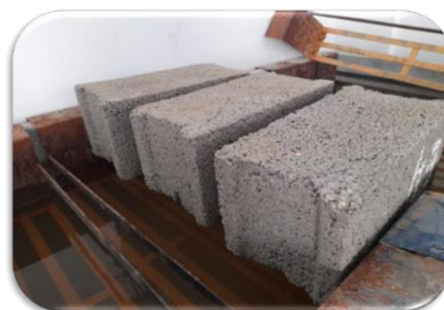
Figure 5: Specimens are removed from water and allowed to drain for 1 min.
