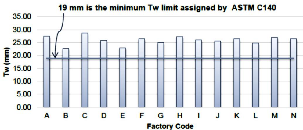
Figure 11: Values of the unit web thickness of average of CMU for all factories.
