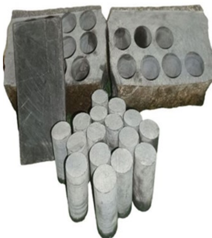
Figure 1: Cylindrical specimens cut from intact blocks of basalt.
