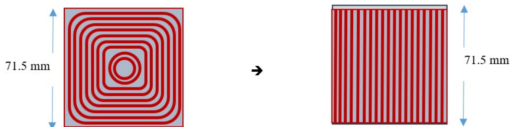
Figure 4: Converting the IRT-4M shape to plates.
