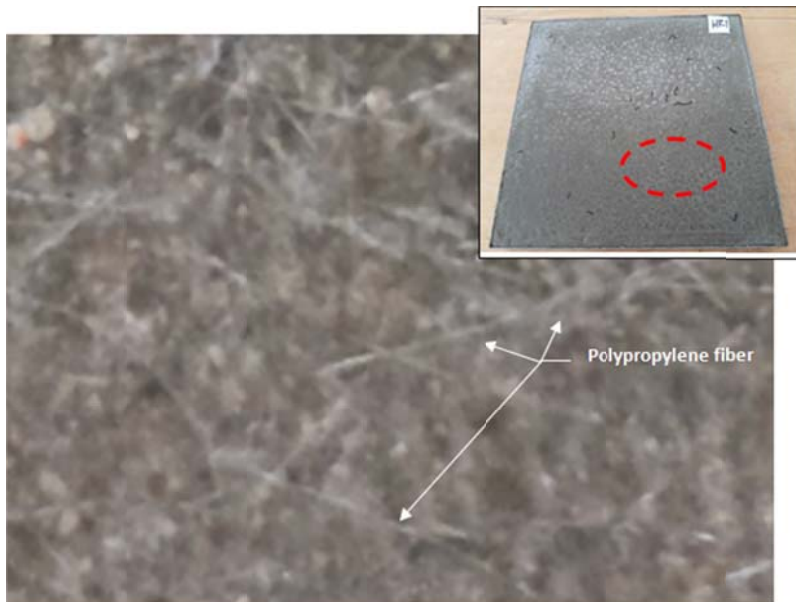
Figure 9: Distribution of fibers on surface of (HF-0.1) concrete slab
