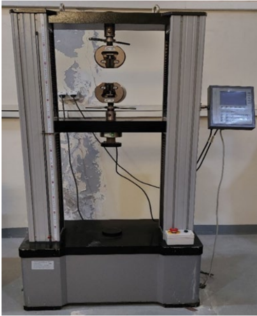
Figure 3: Tensile testing machine at the Advanced Center for Welding, Tajoura, Libya.
